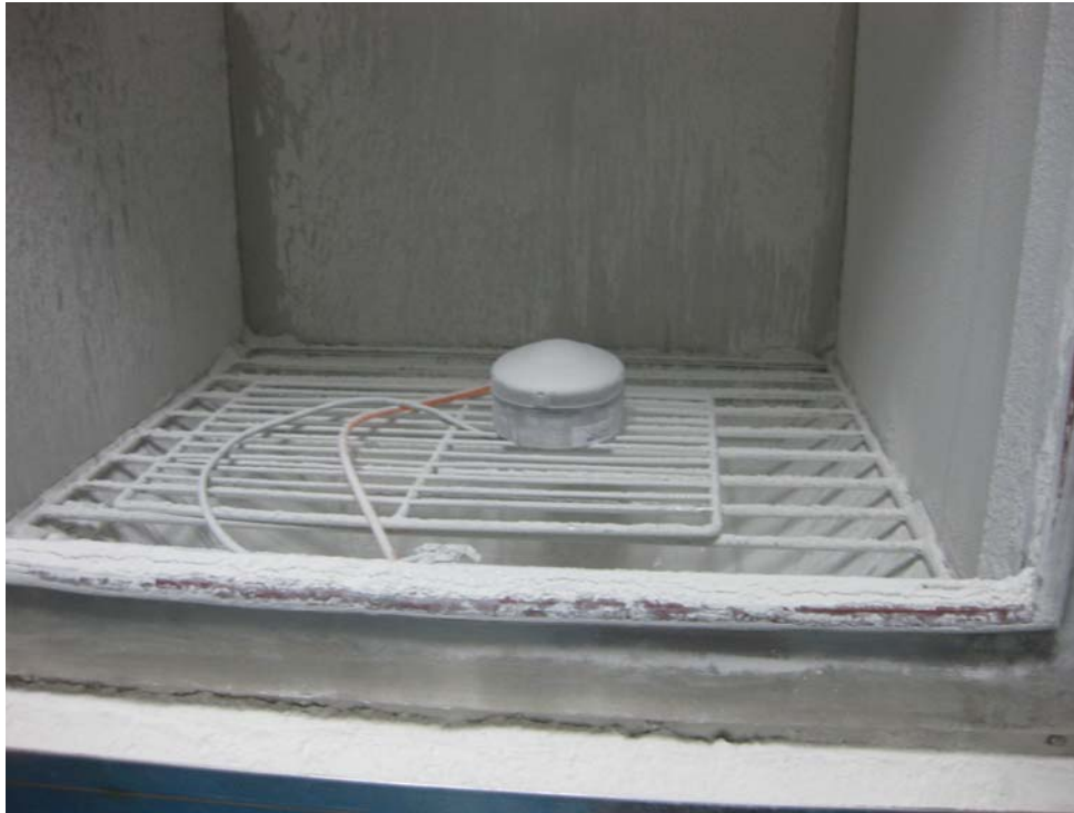
Fig. 3 View after Dust-proof Test
