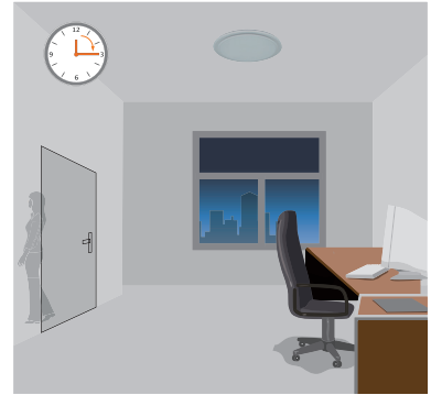
After the hold time, then switches off automatically when no movement is detected.
